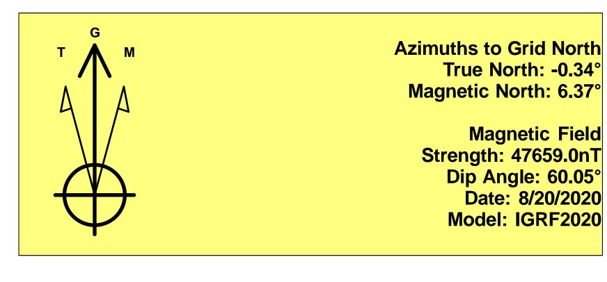
To convert a Magnetic Direction to a Grid Direction, Add 6.37° To convert a Magnetic Direction to a True Direction, Add 6.71° East To convert a True Direction to a Grid Direction, Subtract 0.34°
