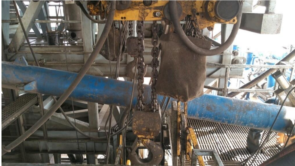
Figure 2: BOP Winch System
