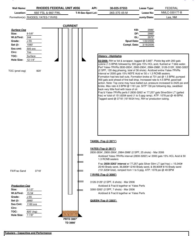
ubing Details: 101 jts 2-3/8" J-55 tbg, SN, 4' perforated sub, 1 open-ended joint of 2-3/8" J-55 tbg; EOT @ 3317.6'
