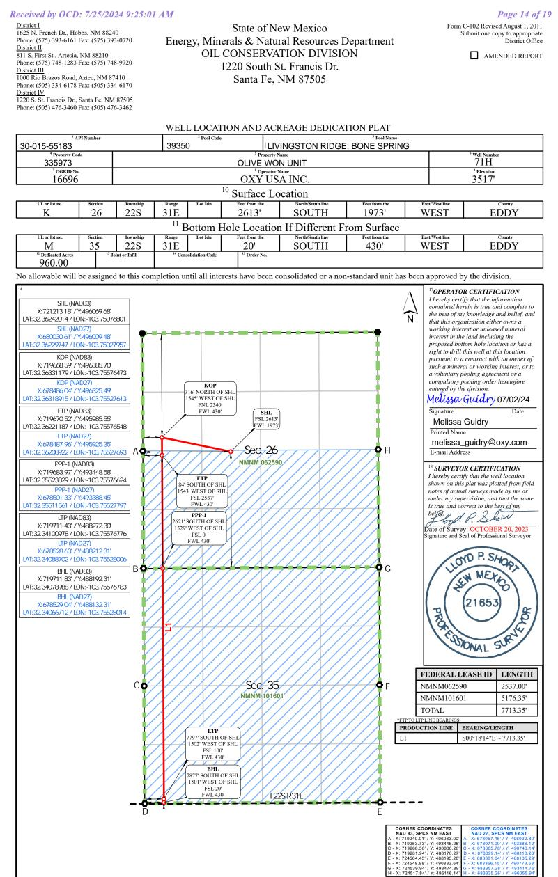
Federal Leases Z HSU OHSU Corners Drill Line Events Section Corners All bearings and coordinates refer to New Mexico State Plane coordinate system, East Zone, U.S. Survey Feet.
