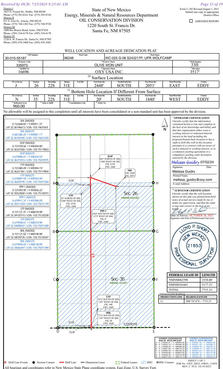
All bearings and coordinates refer to New Mexico State Plane coordinate system, East Zone, U.S. Survey Feet. Distances/areas relative to NAD 83 Combined Scale Factor: 0.99978405 Convergence Angle: 0.31759444° Released to Imaging: 7/25/2024 2:15:51 PM
