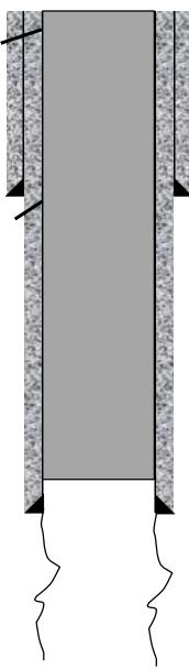
9-5/8" 28 # CASING SET @ 450' IN 12-1/4" HOLE. CEMENT CIRCULATED TO SURFACE W/150 SKS
