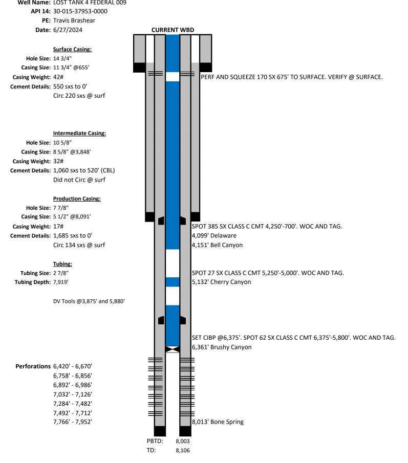
NOTICE OF INTENT TO PLUG AND ABANDON 6/27/2024 LOST TANK 4 FEDERAL 009 30-015-37953-0000 PE: Travis Brashear
