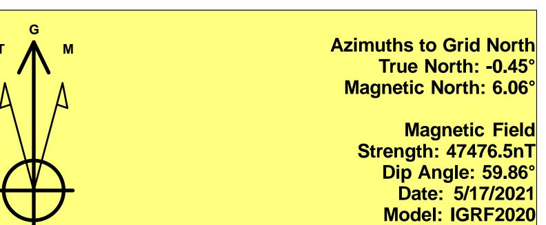
To convert a Magnetic Direction to a Grid Direction, Add 6.06° To convert a Magnetic Direction to a True Direction, Add 6.51° East To convert a True Direction to a Grid Direction, Subtract 0.45°
