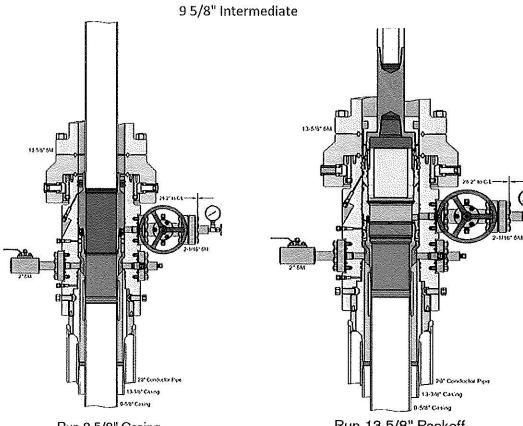
Run 9-5/8" Casing Land Casing on 9-5/8" Mandrel Hanger Cement 9-5/8" Casing Retrieve Running Tool
