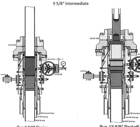
Run 9-5/8" Casing Land Casing on 9-5/8" Mandrel Hanger Cement 9-5/8" Casing Retrieve Running Tool
