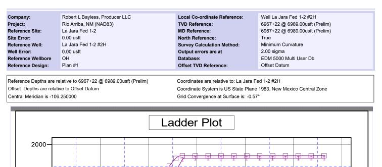
CC - Min centre to center distance or covergent point, SF - min separation factor, ES - min ellipse separation
