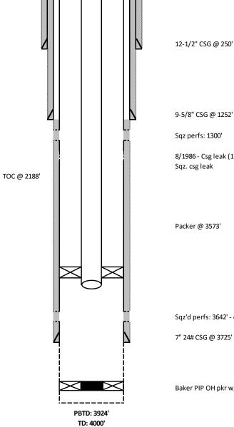
8/1986 - Csg leak (1306' - 16') that held @ 300 psi. NMOCD approved test.
