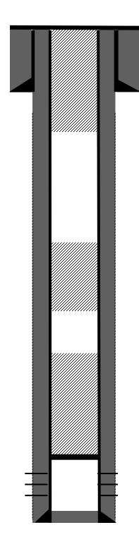
$8\text{-}5/8\sp{"}\,24\sp{\#}\,$  casing @ 145'. Cemented with 150 sks, Class B cement. Circulated cement to surface.
