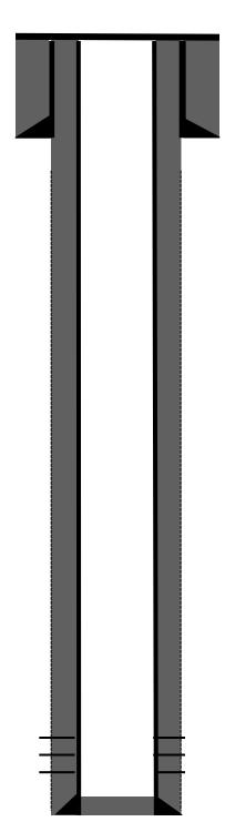
8-5/8" 24# casing @ 145'. Cemented with 150 sks, Class B cement. Circulated cement to surface.
