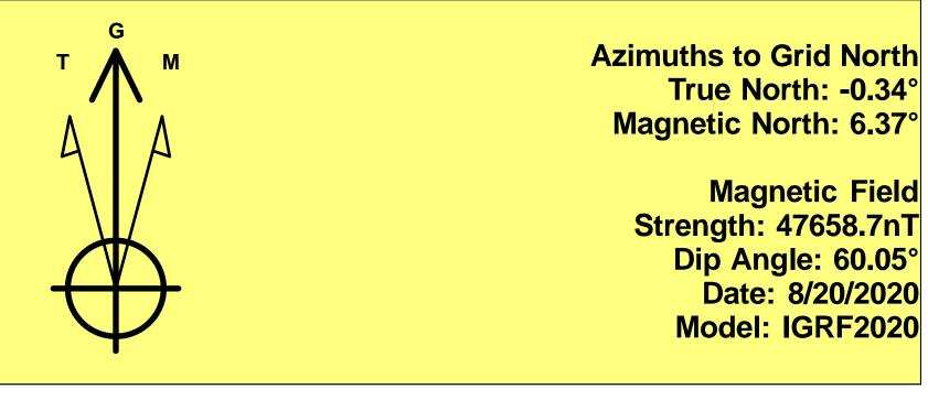
To convert a Magnetic Direction to a Grid Direction, Add 6.37° To convert a Magnetic Direction to a True Direction, Add 6.71° East To convert a True Direction to a Grid Direction, Subtract 0.34°
