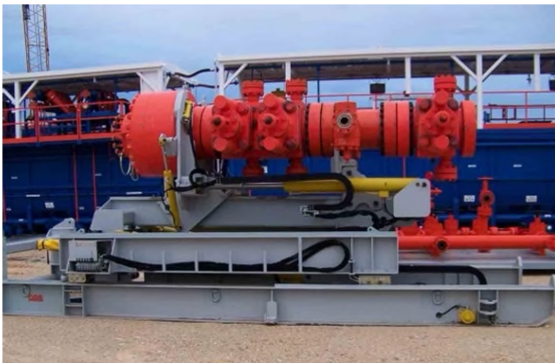
Figure 4. BOP handling system
