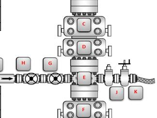
**Pressure Part** Size Description Rating 3" 10,000 HCR (gate valve) 3" K 10,000 Manual HCR (gate valve) Wellhead Pressure **Part** Size Description Rating 13-5/8" 5,000 FMC Multibowl wellhead
