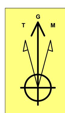
**Azimuths to Grid North** True North: -0.44° Magnetic North: 6.13°
