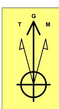
**Azimuths to Grid North** True North: -0.43° Magnetic North: 6.13°
