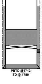
**Plug #1:** Set 5  $\frac{1}{2}$ " CICR @ 1546'. Circ'd hole w/ 40 bbls H2O. Pressure tested csg, held 600 psi. RU wireline. Ran CBL from 1546' to surface. TOC @ 750'. Spotted 18 sx class G cmt w/ 2% CACL @ 1546-1395'. WOC & tagged @ 1380'.
