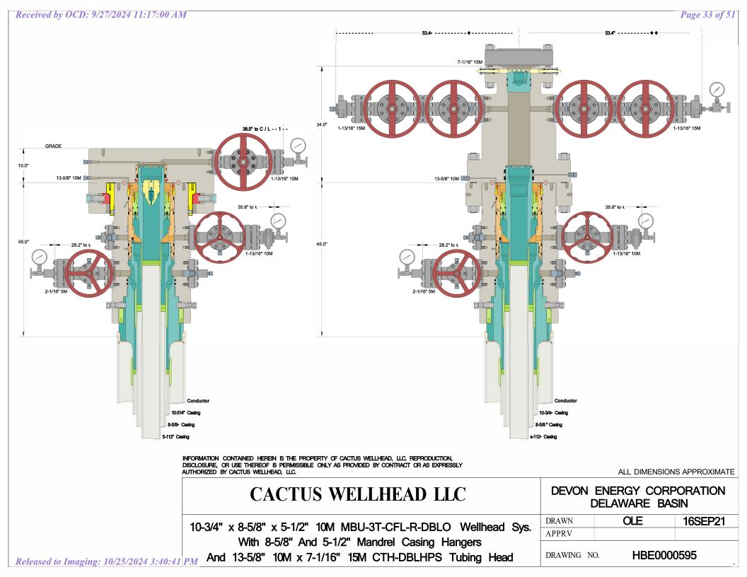
A multibowl wellhead may be used. The BOP will be tested per Onshore Order #2 after installation on the surface casing which will cover testing requirements for a maximum of 30 days. If any seal subject to test pressure is broken the system must be tested.
