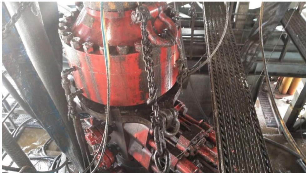
Figure 1: Winch System attached to BOP Stack
