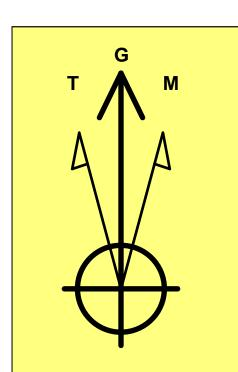
Azimuths to Grid North True North: -0.27° Magnetic North: 6.48°
