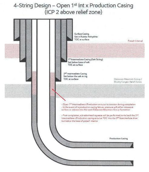
[Figure E] 4 String – Uncemented Annulus between 2<sup>nd</sup> Intermediate and Production Casing Strings
