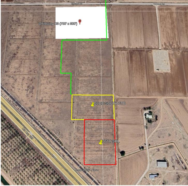
Gas is going to be separated at the Dude South CTB facility – then piped through a low pressure pipe (along the green line) to Enterprise Field Services Whitewing Compressor Station, from there it will go into EFS's system for further processing.
