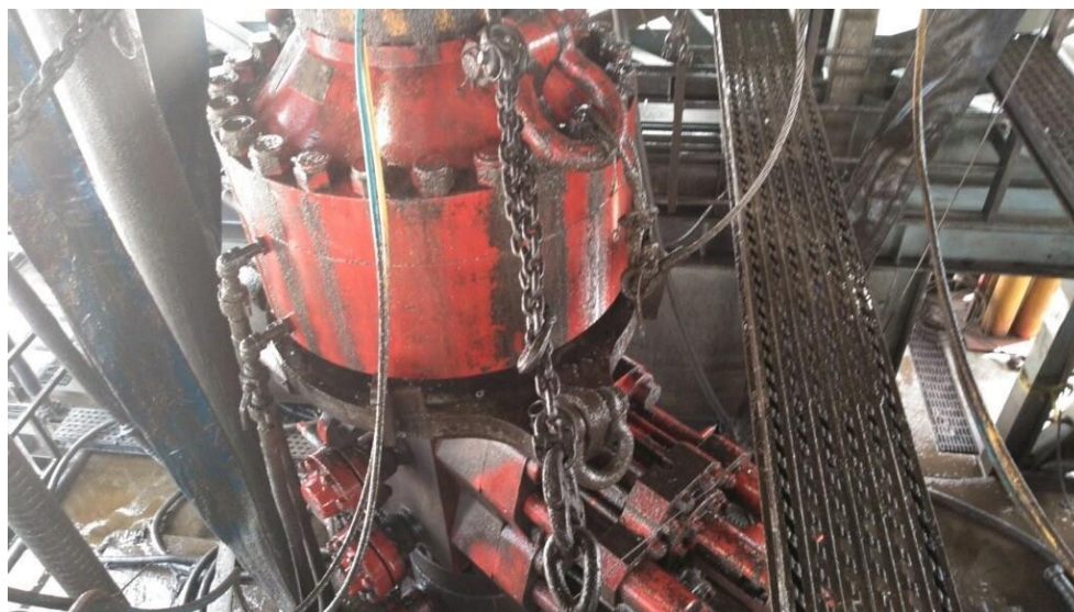
Figure 1: Winch System attached to BOP Stack
