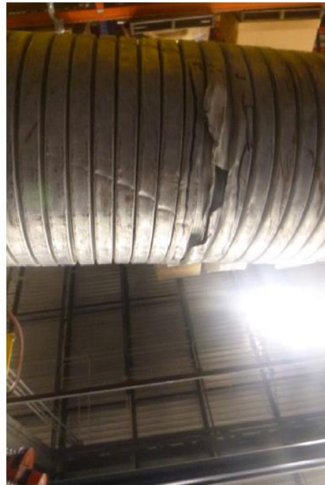
Photo: Damaged armor 11ft 0in. from EF1
