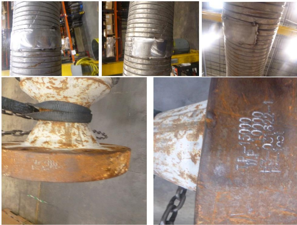
Photos: Repaired Armor and Engraving.
