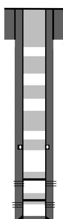
8-5/8" J-55 24# casing @ 217'. Cemented with 140 sks Cement.
