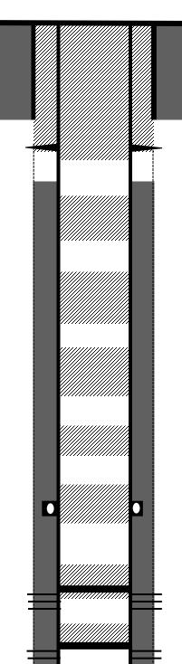
Plug VIII, Inside 4  $\frac{1}{2}$ " casing, Perforations at 260', 76 sks, 87.4 Cu.ft, Surface. 0'-289'
