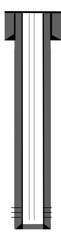
7" 20# casing @ 140'. Cemented with 60 sks, 71 Cu.ft Class B cement. Hole size: 8-3/4". Circulated 4 bbls cement to surface.
