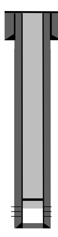
$7"\,20\#$  casing @ 140'. Cemented with 60 sks, 71 Cu.ft Class B cement. Hole size: 8-3/4". Circulated 4 bbls cement to surface.
