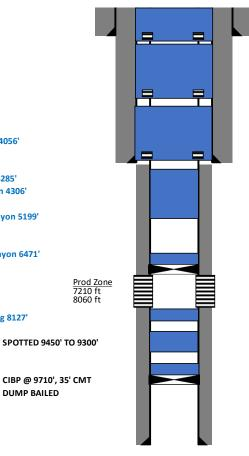
PERF AND CIRC 210 SX CMT FROM 1300' TO SURFACE' **VERIFY CMT TO SURFACE**
