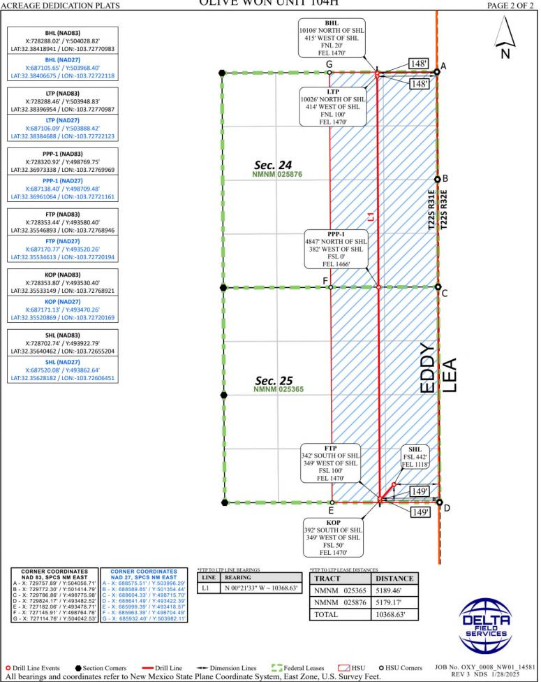
Distances/areas relative to NAD 83 grid measurements. Combined Scale Factor: 0.99978405 and a Convergence Angle: 0.31759200°
