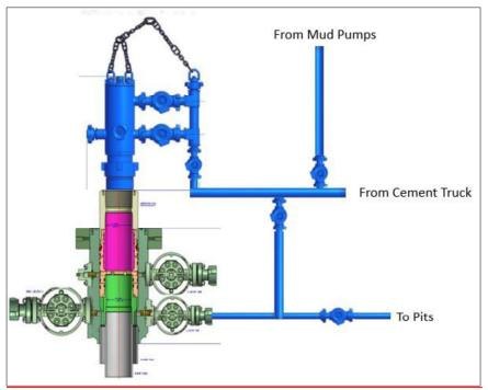
Wellhead diagram during offline cementing operations
