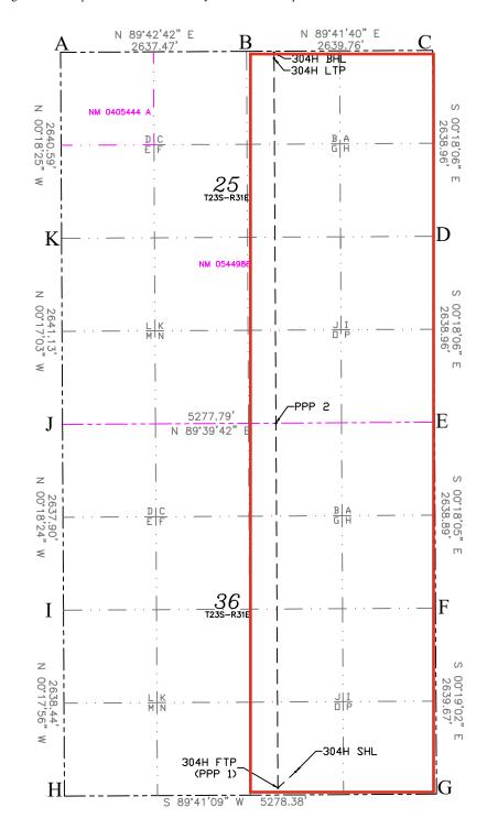
A=N:467082.69 B=N:467095.96 C=N:467110.04 E:724685.21 E:727322.65 E:729962.37 D=N:464471.11 729976.26 E=N:461832.19 F=N:459193.34 729990.15 E:730004.03 G=N:456553.71 E:730018.64 H=N:456524.76 E:724740.34 I=N:459163.17 E:724726.57 E:724712.45 J=N:461801.03 K=N:464442.13 E:724699.35
