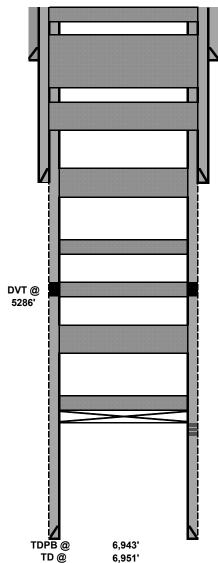
Plug #8: Perf'd @ 100'. Sqz'd 30 sxs class C cmt @ 100' & circulated to surface.
