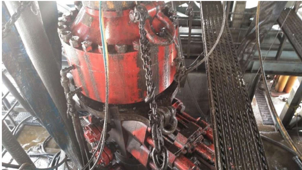
Figure 1: Winch System attached to BOP Stack
