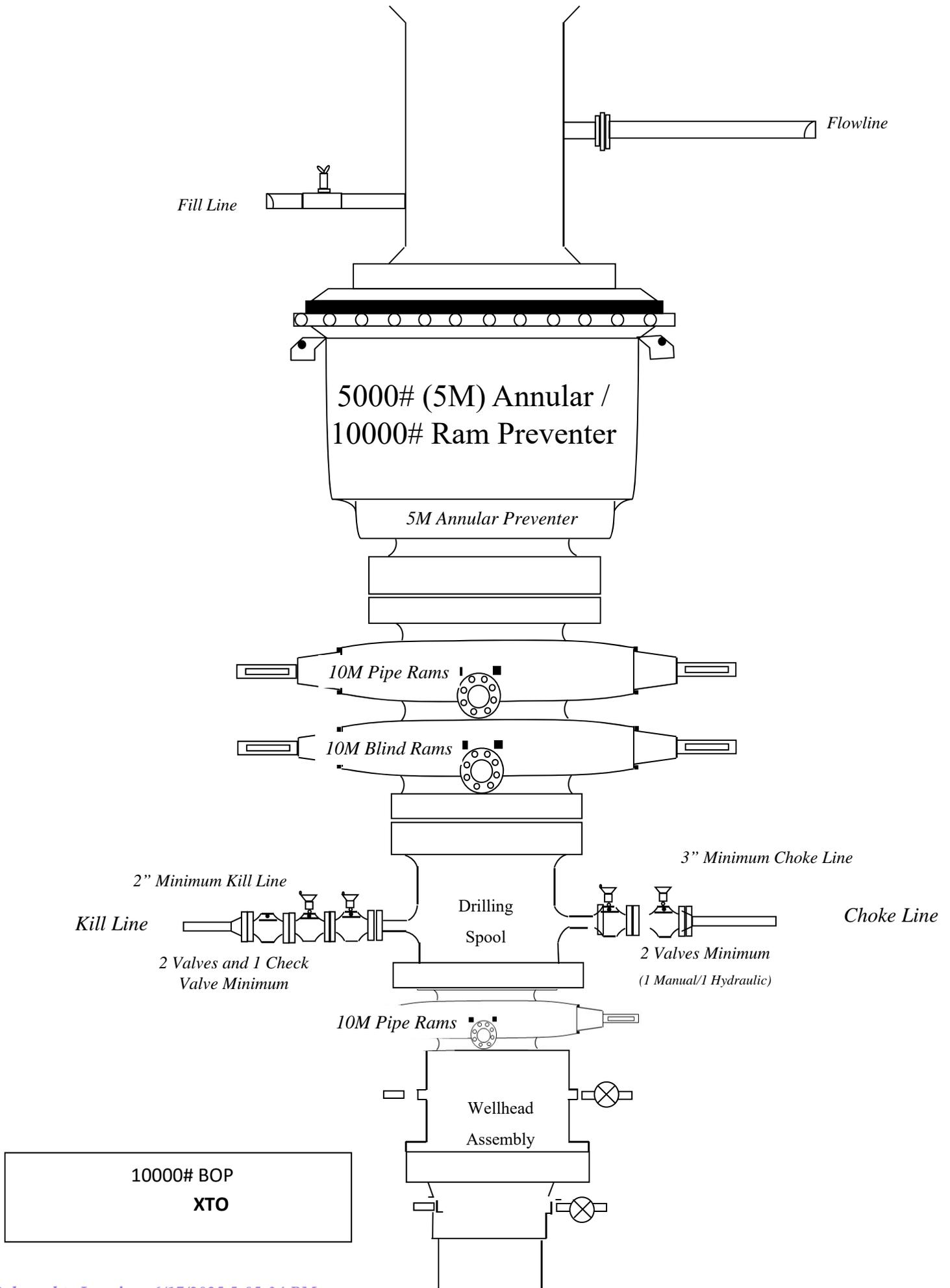
Bleed line will discharge 100' from wellhead for non-H2S situations and 150' from wellhead for H2S situations.
