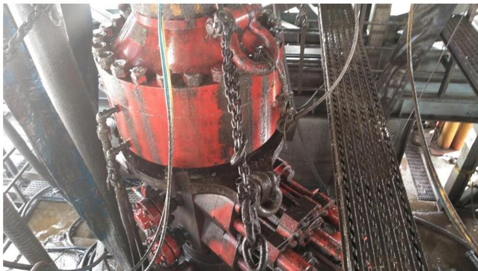
Figure 1: Winch System attached to BOP Stack
