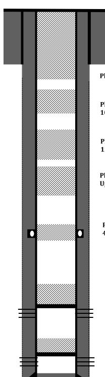
8-5/8" 24# casing @ 334'. Cemented with 225 sks, 260 Cu.ft. Circulated 5 bbls cement to surface
