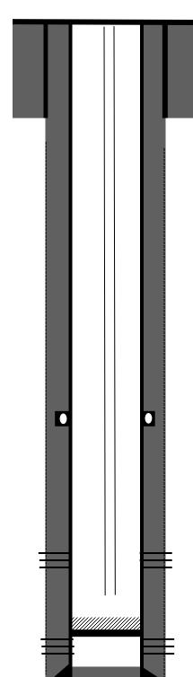
8-5/8" 24# casing @ 334'. Cemented with 225 sks, 260 Cu.ft. Circulated 5 bbls cement to surface
