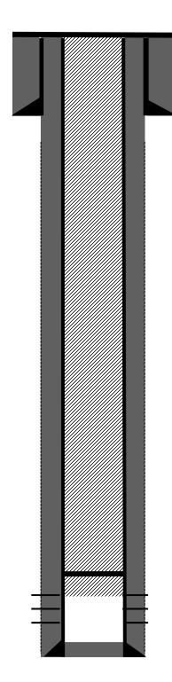
7" 20# casing @ 132' Hole size 9-7/8" Cemented w/ 50 sks Class B neat 2% CaCl2 w ¼#/sk celloflake (59 cu ft). Circ 2 bbls cement to surface
