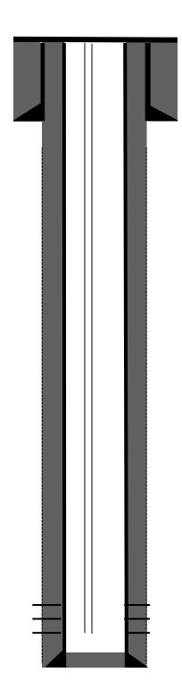
7" 20# casing @ 132' Hole size 8 3/4" Cement w/ 59 cu ft (50 sks) Class B  $\frac{1}{4}$ #/sk cello. Circ 2 bbls cement to surface
