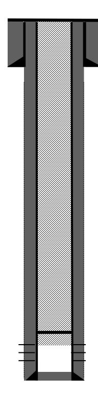
7" 20# casing @ 132' Hole size 8 3/4" Cement w/ 59 cu ft (50 sks) Class B  $\frac{1}{4}$ #/sk cello. Circ 2 bbls cement to surface
