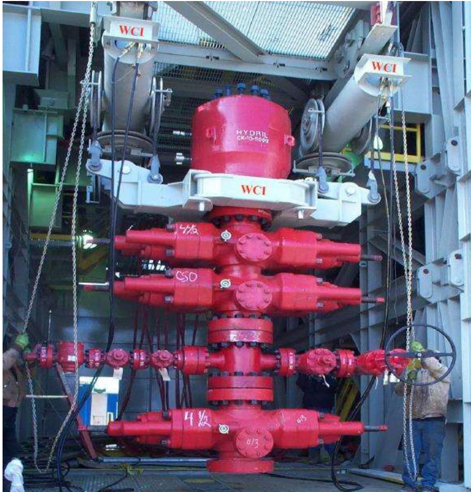
Figure 3. BOP handling system
