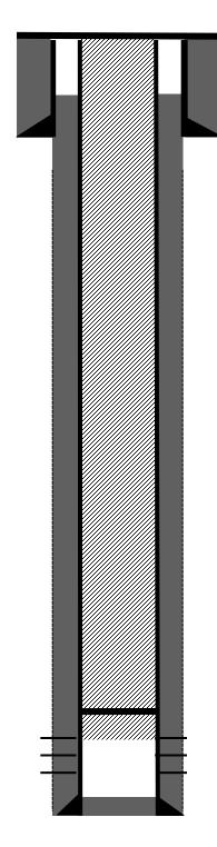
7" 20# K-55 casing @ 125'. Hole size @ 8  $^3$ 4". Cemented w/ 70 sks (83 cu ft) Class B cement. Circulated 4 bbls cement to surface.
