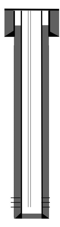
7" 20# K-55 casing @ 125'. Hole size @ 8  $\frac{3}{4}$ ". Cemented w/ 70 sks (83 cu ft) Class B cement. Circulated 4 bbls cement to surface.
