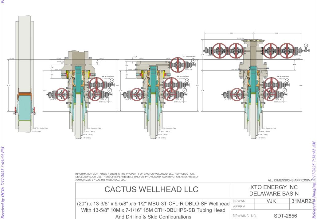
And Drilling & Skid Configurations
