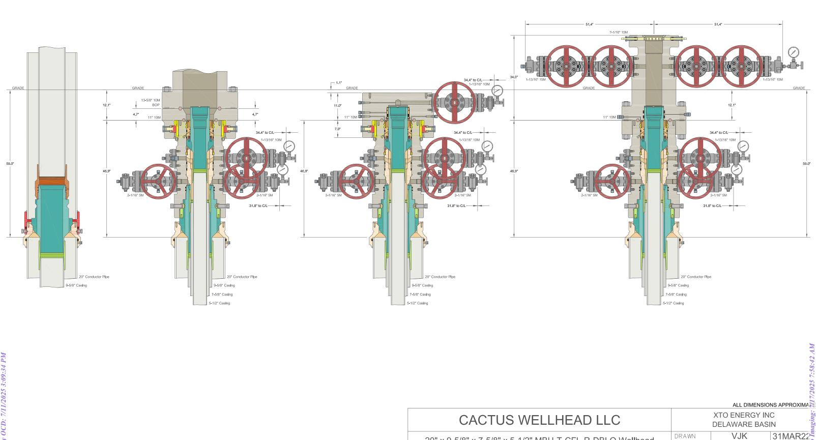
20" x 9-5/8" x 7-5/8" x 5-1/2" MBU-T-CFL-R-DBLO Wellhead With 11" 10M x 7-1/16" 15M CTH-DBLHPS Tubing Head And 9-5/8", 7-5/8" & 5-1/2" Pin Bottom Mandrel Casing Hangers
