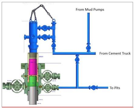
Wellhead diagram during offline cementing operations
