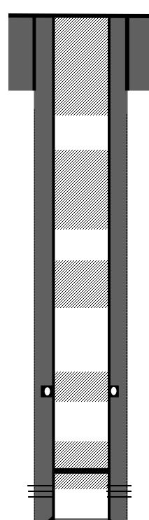
8 5/8" 24# casing @ 225'. Spud hole 12  $\frac{1}{4}$ " Cemented with 117 cf 160sks Class B w 2% CacL  $\frac{1}{4}$  #/sk Flocele.
