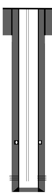
$8\,5/8"$  24# casing @ 225'. Spud hole 12 ¼" Cemented with 117 cf 160sks Class B w 2% CacL ¼ #/sk Flocele.
