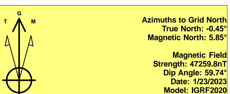
To convert a Magnetic Direction to a Grid Direction, Add 5.85° To convert a Magnetic Direction to a True Direction, Add 6.30° East To convert a True Direction to a Grid Direction, Subtract 0.45°
