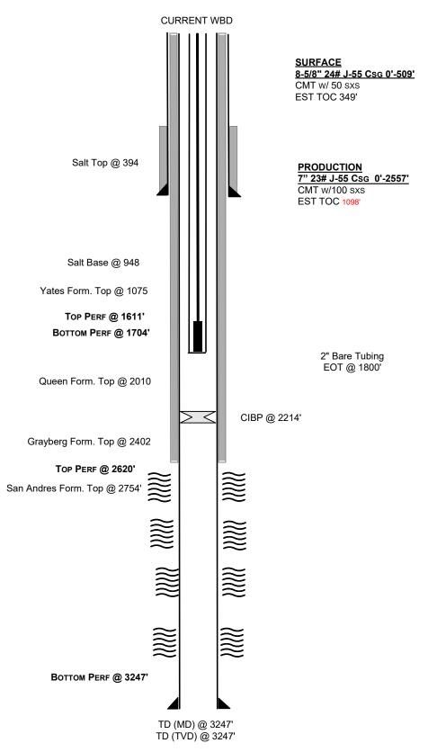
EVENT LOG 6/4/50-DRILLED WELL 8/3/50- COMPLETED WELL- OH COMPLETION 2620-3247 7/22/55- RECOMPLETED WELL 8/9/74- SET CIBP AT 2214, THEN PERF 1611-1704
