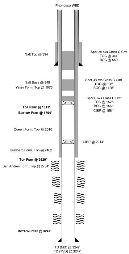
EVENT LOG 6/4/50-DRILLED WELL 8/3/50- COMPLETED WELL- OH COMPLETION 2620-3247 7/22/55- RECOMPLETED WELL 8/9/74- SET CIBP AT 2214, THEN PERF 1611-1704
