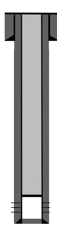
8-5/8" 23# casing @ 126'. Cemented with 88 Cu.ft Class B cement. Hole size: 11". Circulated 3 bbls cement to surface.
