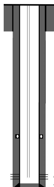
$8\,5/8$ " 24# casing @ 194' Hole size  $12\,\frac{1}{4}$ " Cement w/ 135 sks class B. Circ cement to surface
