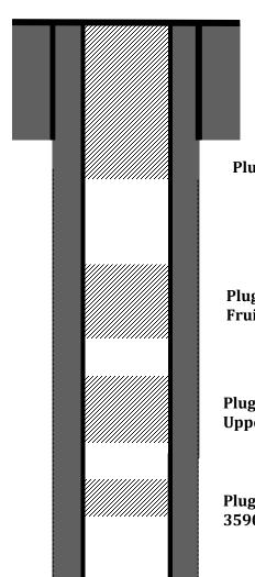
$8\,5/8$  " 24# casing @ 194 ' Hole size  $12\,\frac{1}{4}$  " Cement w/ 135 sks class B. Circ cement to surface
