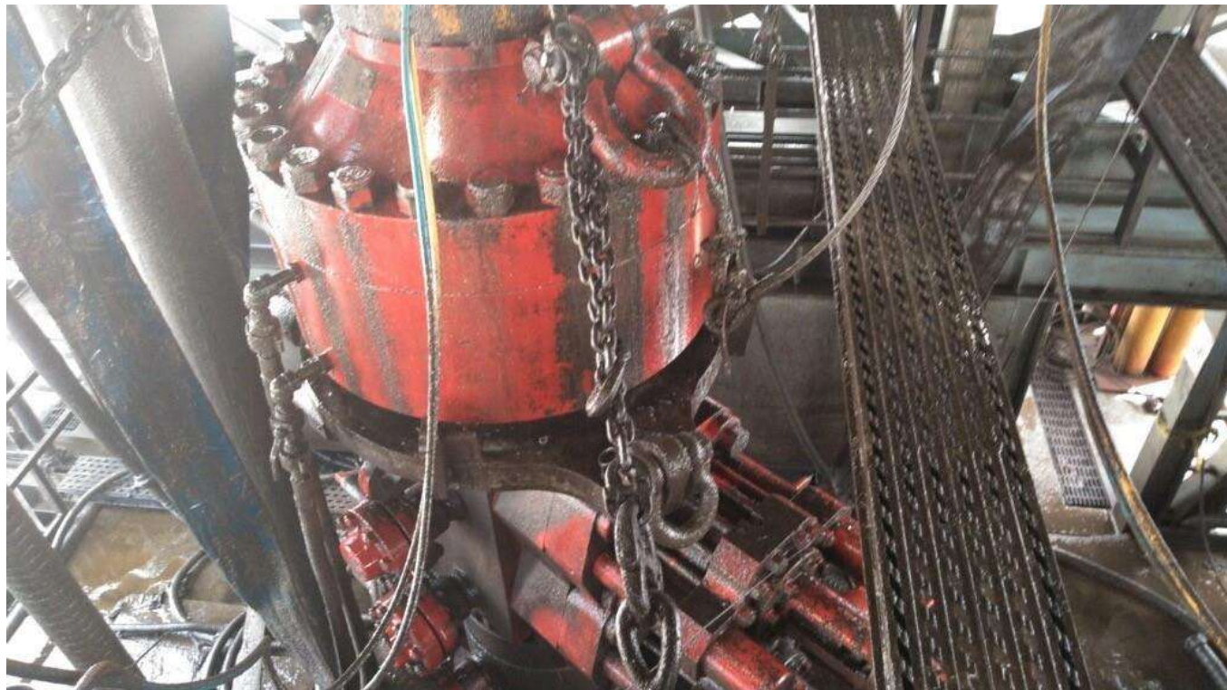
Figure 1: Winch System attached to BOP Stack
