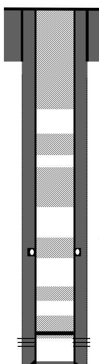
Hole 12 ¼", Casing 8-5/8" 24# @ 259' Cemented w/ 150 sks Class B. Cement circulated.
