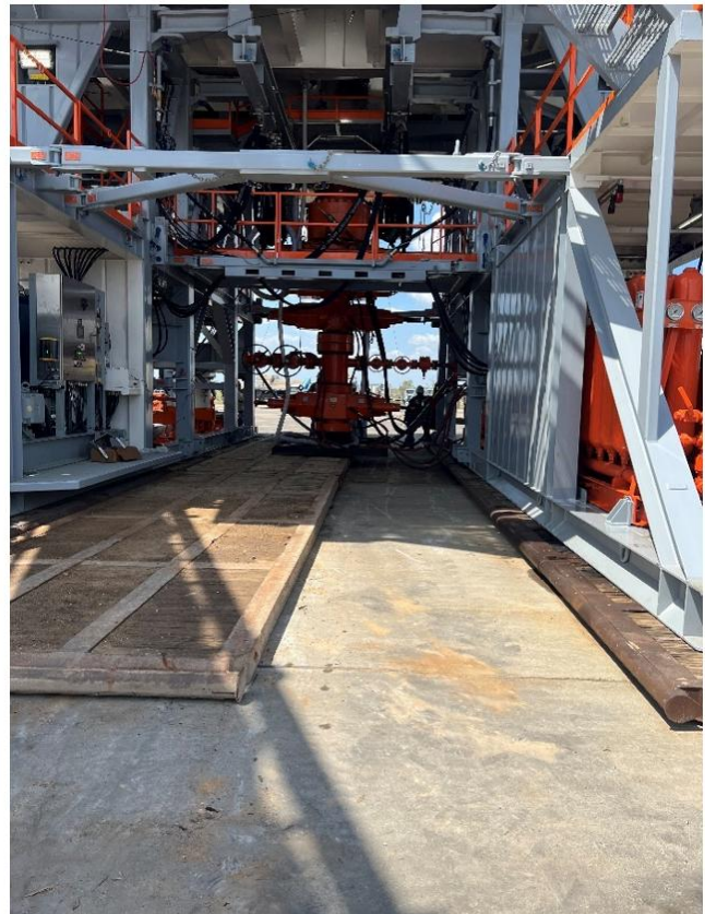
Figures 1 & 2: BOP winch system picture with walking capabilities.
