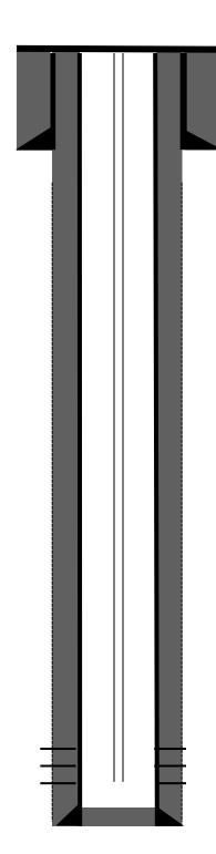
**8-5/8" 24#, J-55 casing @ 136': Hole size - 12 ¼"**Cemented with 100 sks, Class G cement. Circ 4 bbls cement
