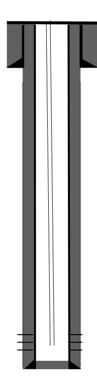
**8-5/8" 24#, J-55 casing @ 131': Hole size – 12 ¼"**Cemented with 100 sks, Type 5 cement. Circ 4 bbls cement
