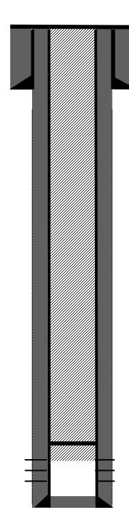
**8-5/8" 24#, J-55 casing @ 131': Hole size – 12 ¼"** Cemented with 100 sks, Type 5 cement. Circ 4 bbls cement
